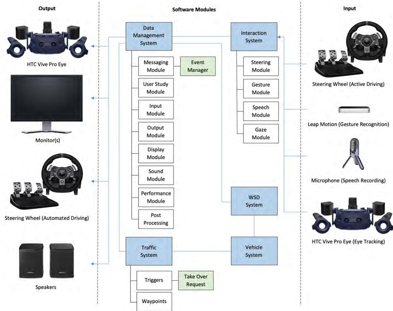
**Figure 5:** Graphic representation of the various architectural components constituting the AutoWSD driving simulator.
