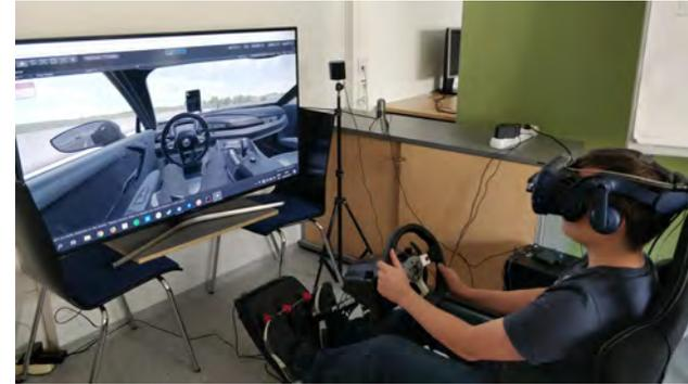
**Figure 4:** Demo setup with a virtual reality head-mounted display, steering wheel and 4K screen.
