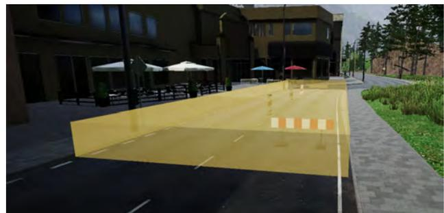
Figure 3: Take over request trigger, displayed in yellow, for triggering a manual take over because of an unexpected road situation.
